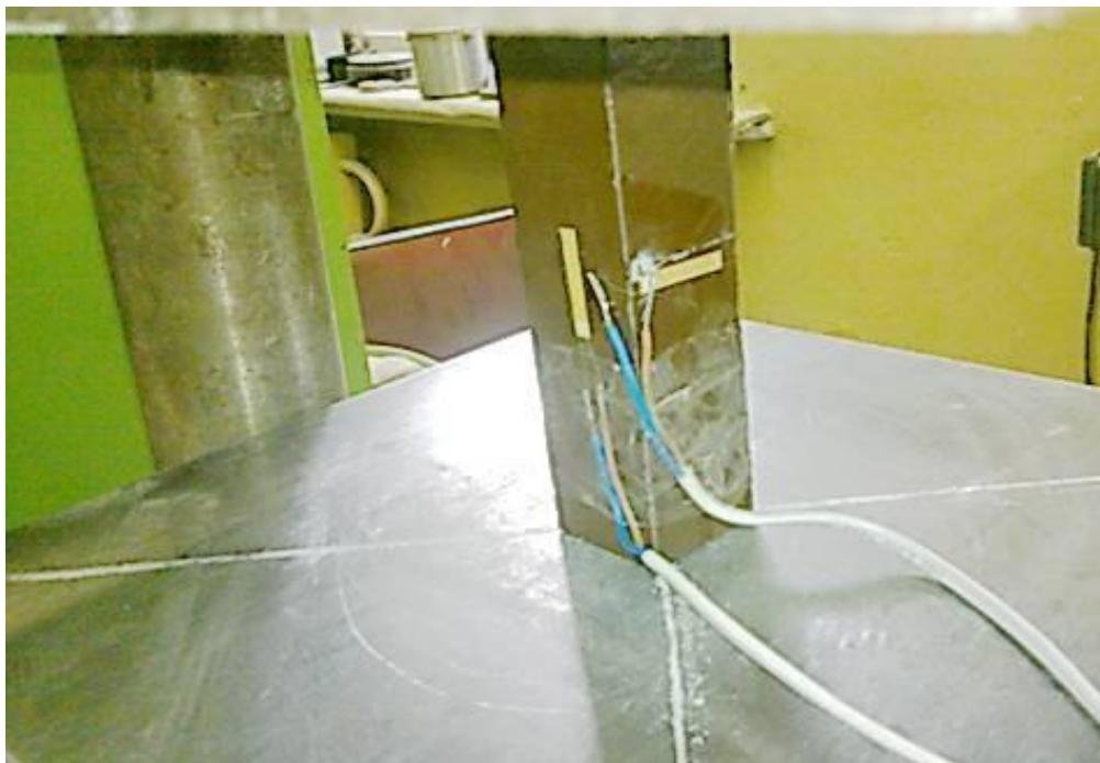
Figure 1 : Scheme of installation of strain gauges for testing specimens for compression
